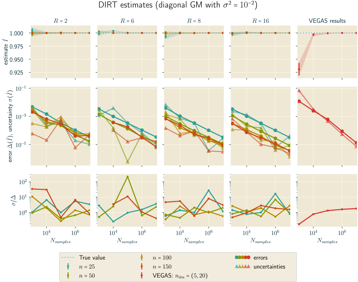
Figure 4.6: Varying the number of samples N for different numbers of initial TT-ranks R_0 and g(\vec{x}; \vec{\mu}_i, \sigma^2 = 10^{-2}) .
