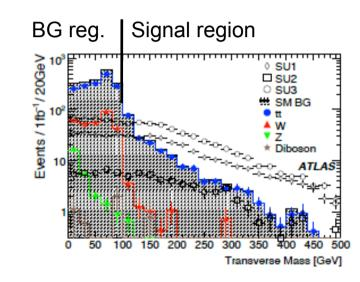
the fitting method can be used: SUSY contamination in CS is estimated from Signal region with assumption SUSY MT distribution is flat. It works, but depends on model.
